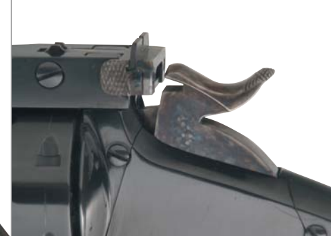
HALF COCK POSITION OF THE HAMMER
